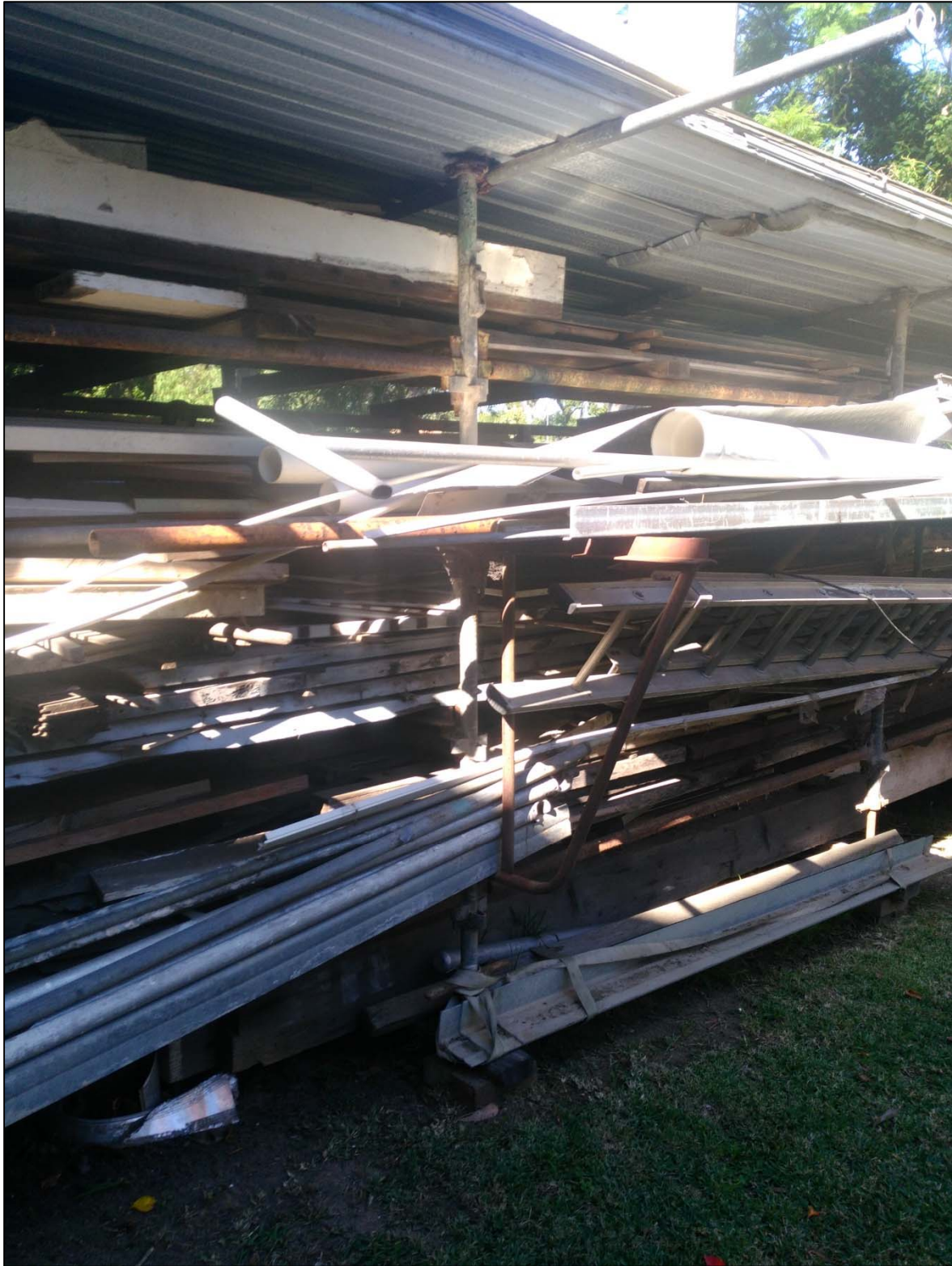
Photograph 6: Stockpiled building materials found on a residential property on the northern side of the site (Chapman Avenue); the pile may be susceptible to weathering processes, which in turn may lead to a localised source of subsurface contamination (i.e. leached metals).
